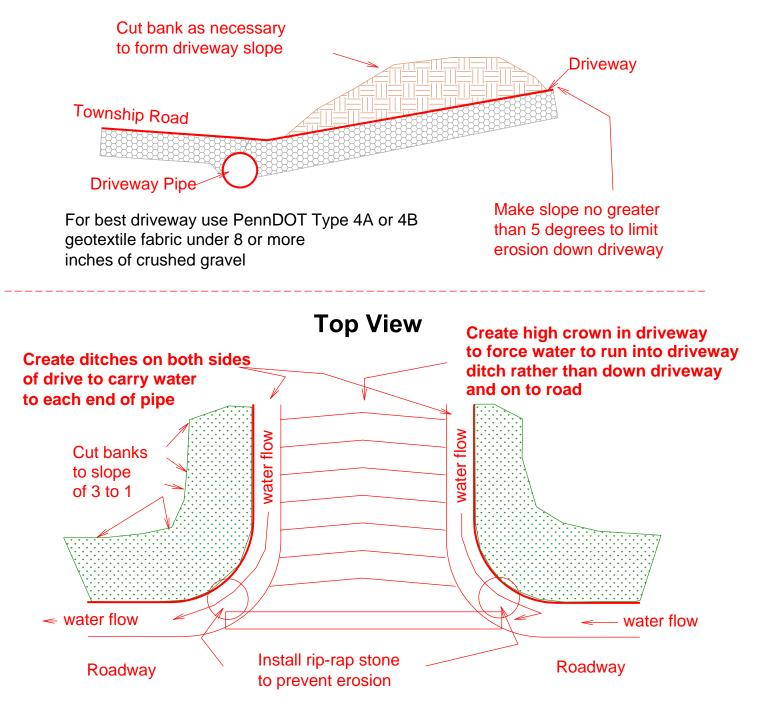
Driveways that run uphill from the road require constant maintenance by the landowner. Failure to keep a high crown in the drive and clean, deep ditches along the drive will result in significant erosion of the driveway gravel during heavy rain storms. More importantly, water will run down the drive in winter and freeze on the road creating a dangerous ice condition. This may result in the landowner being liable for damages from an accident created by the ice condition.
